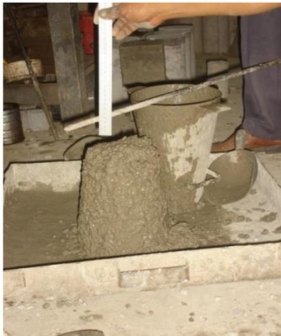
**Gambar 4.** Uji *slump* beton
